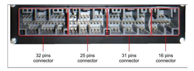
The connector to be used for CAN Connection is the 31 pins. It is shown here below: please note that pins are to be numbered from right to left in each row.
