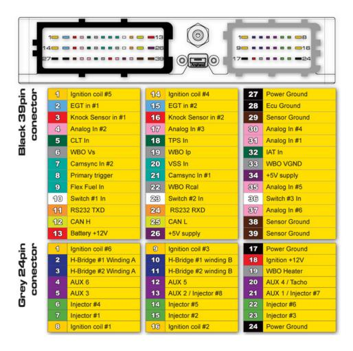
RS232TX: pin 11; 39 pins connector (Black) RS232RX: pin 24; 39 pins connector (Black)
