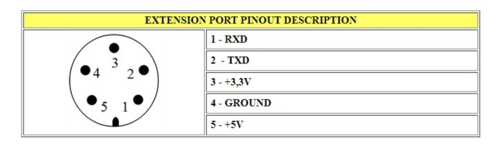
**Please note**: with serial communication protocol it is mandatory to connect ECU GND with AiM device GND as well as ECU TXD is to be connected to AiM ECU RS232 TX (or AiM RS232RX for older products) and vice versa.
