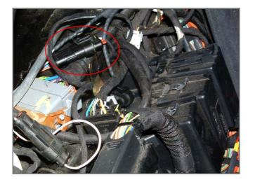
4 pins Superseal connector pin
