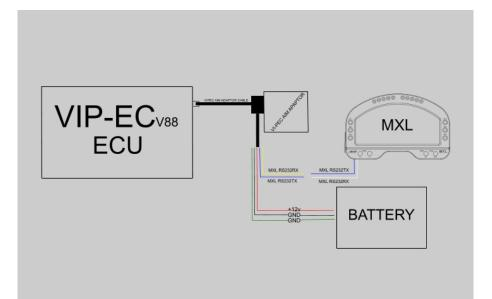
Note: for the ECU to correctly communicate with AIM loggers it is necessary to connect both devices to Vi-PEC-AIM adaptor, supplied with the ECU, that takes bit rate to 19200 bps.
