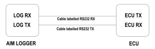
Vi-PEC ECU data transmission is 57600 Baud, for this reason Vi-PEC has created "Vi-PEC AIM ADAPTOR" that converts and re-transmits data at 19200 baud.
