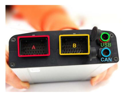
"A" connector is necessary to power the ECU
