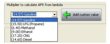
In case used fuel is not included in the database and **only in case its Stoichiometric value is known** press "Add custom value" button and the window shown below appears.
