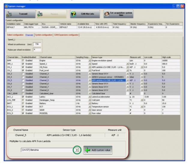
Activate the drop down menu pressing the arrow button circled in the image above and select the fuel used by the vehicle.
