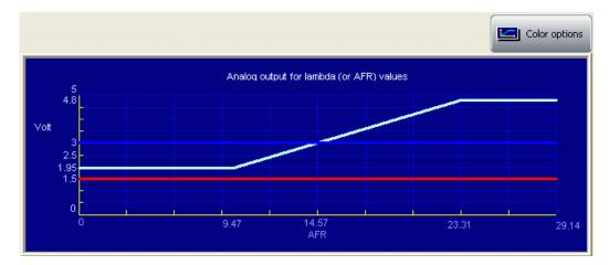
The "analog output graph" shows output tension values of the controller in correspondence of the measured Lambda values. Graph colours are customizable. Pressing "Colour options" button the window shown below appears:
