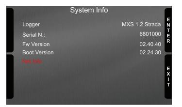
"Net info" option appears only if an expansion is connected to MX Strada, GPS included and pressing "ENTER" button the information of these expansion are shown as below.
