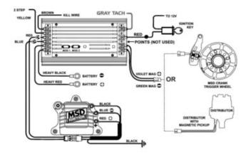
The output labelled "GRAY TACH" gives a 5-50V output that can be directly sampled by MX Strada series dash.
