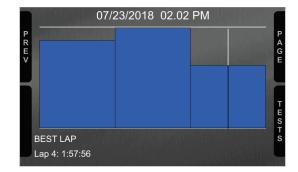
Third is "Summary" page that shows all tests in a box with time of the test, number of laps and best lap of the test. Select the test to see and press "ENTER".
