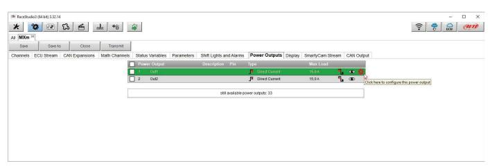
The setting panel appears: fill it in. In the example Power output 1 has been configured to manage a fan: it turns ON when Water temperature is greater than 90°C: Max accepted current (Maximum value of requested Loan) is 8 Amp: over this value the output circuit opens and the read status becomes "Overcurrent".
