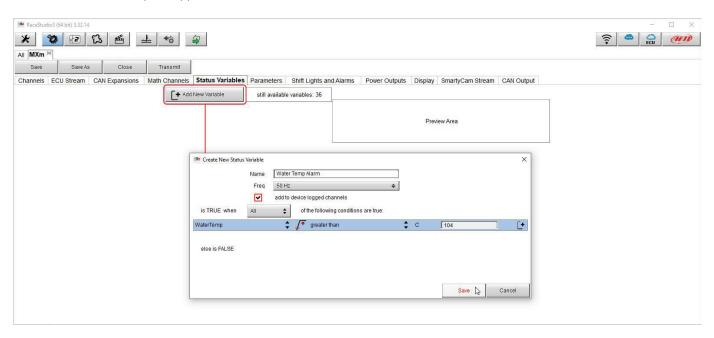
In the example below the user created a Status variable called "Water Temp Alarm". Mousing over the status variable row a summary panel appears on the right while mousing over each square of the row a popo up explains its meaning.
