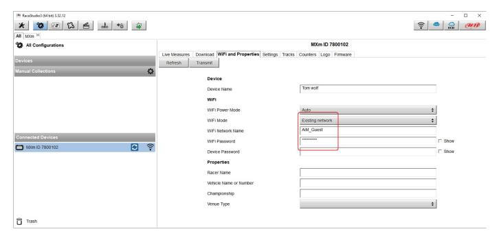
Here above you see a device "MXm ID 6500100" that switched from AP to WLAN mode (Existing Network).
