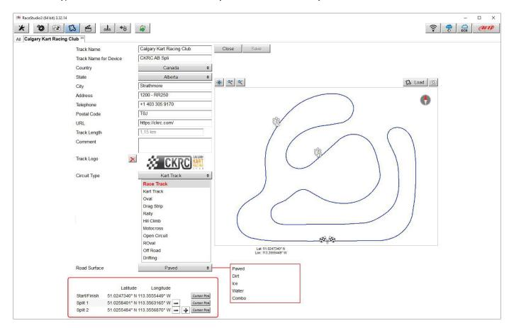
It is possible to change the start line position (move the cursor and set "Cursor Position") and to add split points in order to organize the track in different segments. This will be used in Data Analysis.
