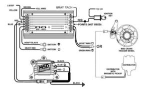
The output labelled "GRAY TACH" gives a 5-50V output that can be directly sampled by MXm.
