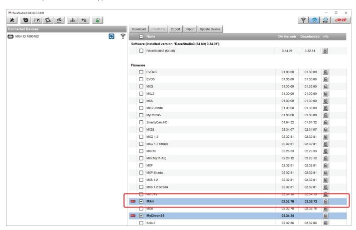
Once the new firmware has been downloaded connect your device to the PC via Wi-Fi to perform a firmware upgrade. In a few seconds the device is ready.
