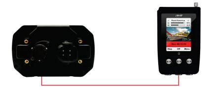
To connect MXm to LCU-One CAN connect cable labelled "EXP" of MXm 37 pins connector harness to 5 pins Binder connector of LCU-One as shown here below.
