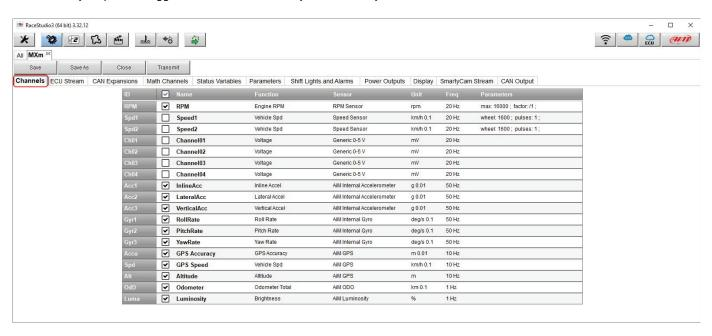
To set a channel just click on its line and the related panel shows up. Speed 1 and 2 and the four Analog channels are disabled by default. First thing to do is enabling them.
