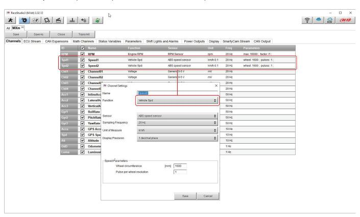
To set the four **Analog channels** click on the related row, a setting panel appears and you can choose function, sensor type, measure units, display precision or specific parameters.
