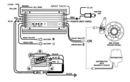
The output labelled "GRAY TACH" gives a 5-50V output that can be directly sampled by MX Series logger.
