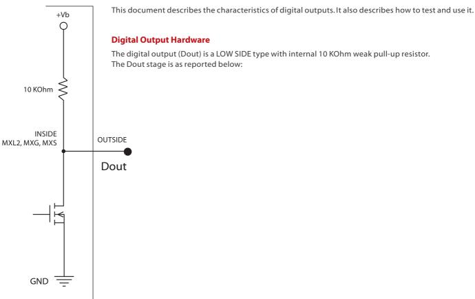
The digital output (Dout) is a LOW SIDE type with internal 10 KOhm weak pull-up resistor.
