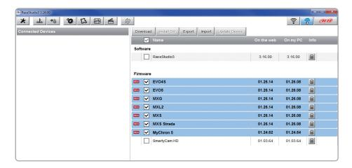
Once the new firmware has been downloaded, connect your device to the PC via Wi-Fi to perform a firmware upgrade. In a few seconds the device is ready.
