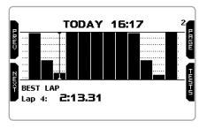
This page shows the selected lap with max/min RPM and speed values
