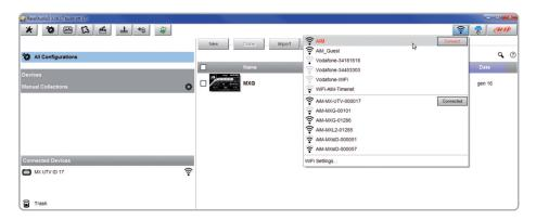
When the PC is authenticated to the network called "AiM" it can see all devices you configured to access the same network. In the image below two AiM devices are connected to the same "AiM" WLAN.
