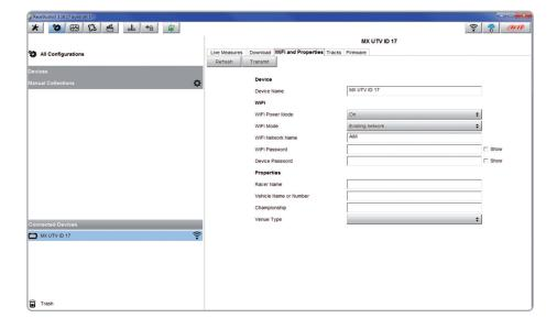
Here above you see a device "MX UTV ID 017" that switched from AP to WLAN mode ("Existing Network").
