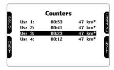
Each odometer can be activated/deactivated and/or reset. Select the odometer you want to manage and press "CHANGE":
