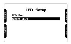
In this page (left image below) you can link each LED to one of the channels supplied by your vehicle ECU. As you see in addition to the usual ECU channels, MX UTV supplies three average belt temperatures, to say:
