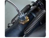
"Do not run the RPM lead in any type of tubing; it should be run right along the frame rail.
