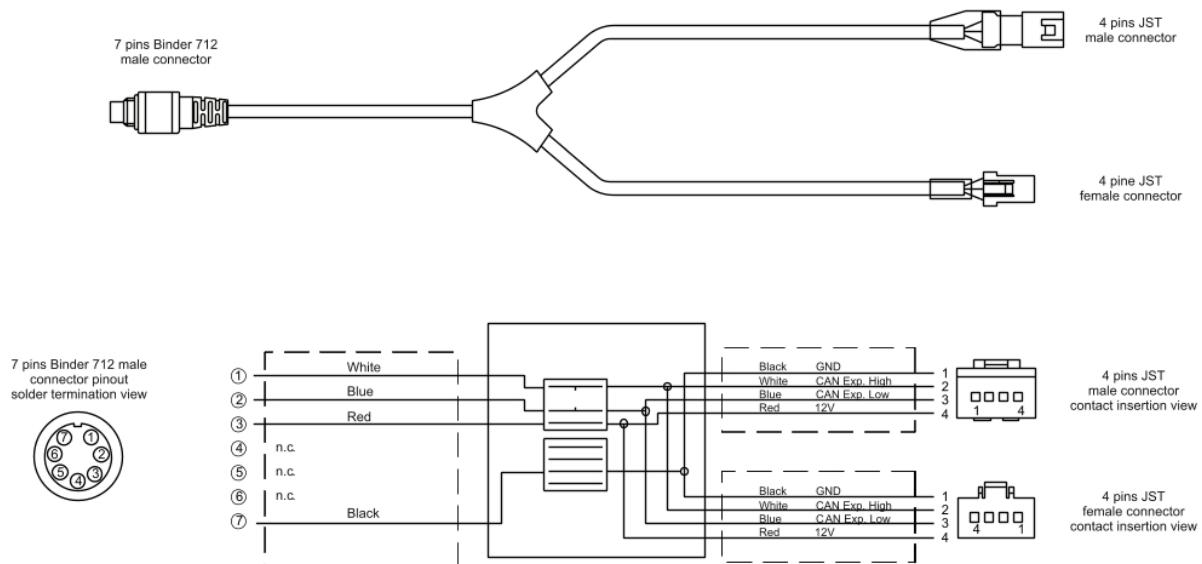
The image below shows the connection scheme of AiM Taipan ECU and Solo 2 DL.
