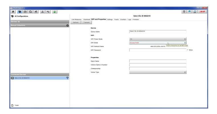
This AP or SSID name is unique for your device. An example of name is:" AiM-Solo2DL-00103" where:
