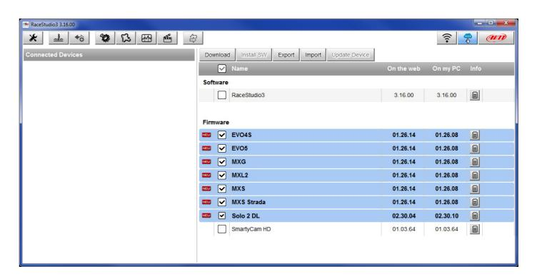
Once the new firmware has been downloaded connect your device to the PC via Wi-Fi to perform a firmware upgrade. In a few seconds the device is ready.
