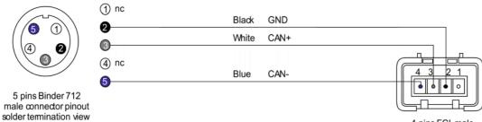
4 pins FCI male connector pinout contact insertion view
