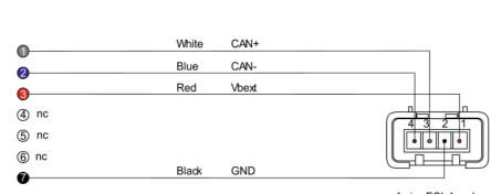
4 pins FCI 4 male connetor pinout contact insertion view
