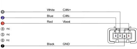
4 pins FCI 4 male connetor pinout contact insertion view
