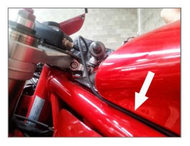
Connect the cable to SoloDL as here on the right.
