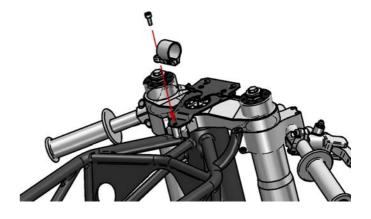
Replace the stem in the collar re-screwing its screws and replace Uniball screw fixing it to the frame pivot.
