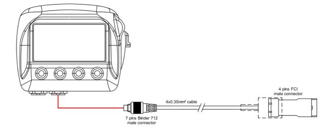
To connect AiM EVO4 to **V02563150** cable use the five pins Binder 712 female connector labelled "ECU" of the logger – third from the left on the top row –as shown here below.
