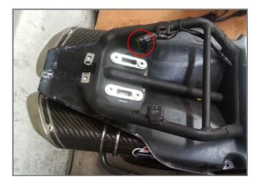
Once the cup has been removed the connector appears as here on the right.
