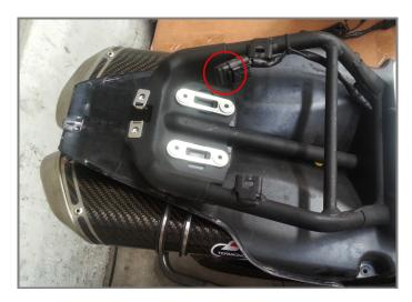
Once the cup has been removed the connector appears as here on the right.
