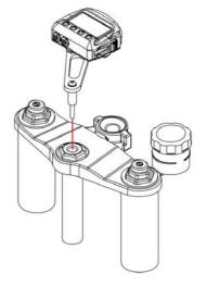
Tighten the central screw on the hinge so that the rawl nut grips.
