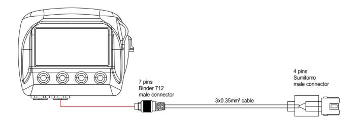
As said SoloDL connection kit allows also to power the logger. The table below shows colours of the cables connected to Honda Sumitomo connector and their function.
