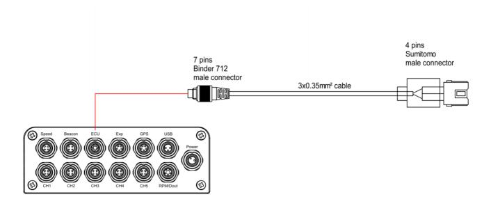
As said EVO4S connection kit allows also to power the logger. The table below shows colours of the cables connected to Honda Sumitomo connector and their function.
