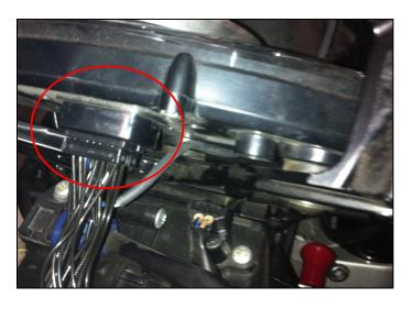
If you installed **EVO4**, take AiM cable – highlighted in the image – to it. If you installed a **SoloDL** make AiM cable pass around the bike stock dash.
