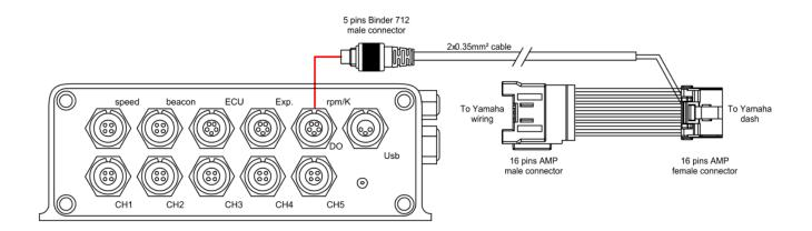
Connection between AiM EVO4 and Yamaha YZF-R1 2009-2014 (cable with JAE connectors) is shown here below.
