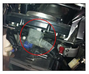
Remove the rubber cover from the connector as in the image.
