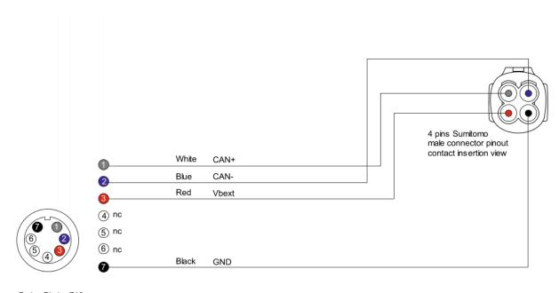
7 pins Binder 712 male connector pinout solder termination view
