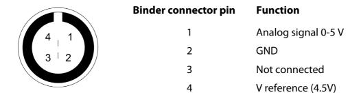
The car/bike linear potentiometer **electrical characteristics** are:
