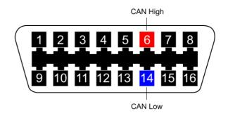
OBDII connector pinPin functionAiM cable6CAN HighCAN+14CAN LowCAN-
