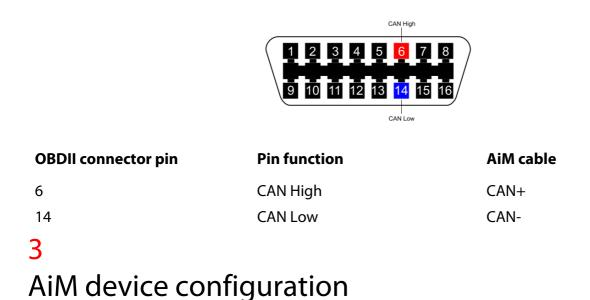
Before connecting the ECU to AiM device set this up using AiM Race Studio software. The parameters to select in the device configuration are:
