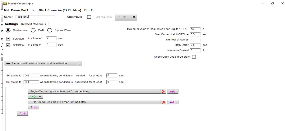
It is also possible to have the fan controlled by a PWM (pulse with modulation) output which for example could start at 40C with 30% of power and have 60% power at 60C and go to 100% power at 85C. In all these cases the fan will lose power if the car is traveling in excess of 60mph.
