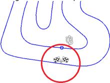
Another reason is relevant to optic receivers, in particular when more transmitters are placed on the pit wall and the logger triggers more than one signal. In this case, the solution is supplied by the obscuring time you can set with the "Ignore additional lap signal for XXX sec".
