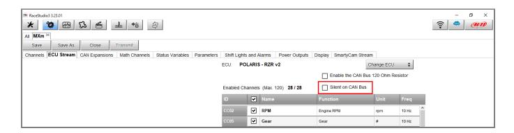
The Silent Mode disabling (default setting) activates the Acknowledge bit management, which indicates the presence of errors (NACK) or the absence of anomalies (ACK). Ticking the proper box, the system is set as Silent, not managing the above described bit.
