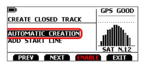
Solo2/Solo2DL automatically creates a track and, once the session is over, the new track layout is displayed; the start/finish line can be changed, and a track name can be added using the device keyboard. You may transmit the track information to your PC and, by Race Studio 3, modify its details.
