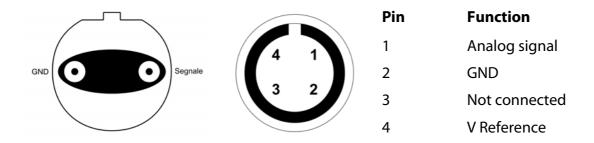
The table here below shows the sensor electrical characteristics.
