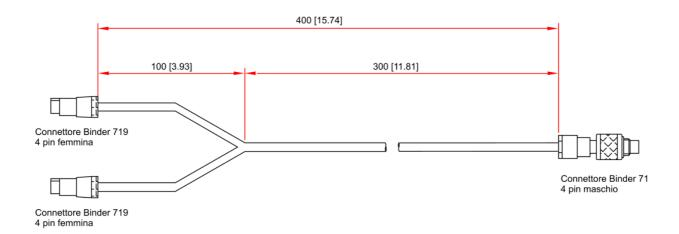
The sensor has a cable ending with a 4 pins Binder (719 or 712) male connector. The table below shows the connector – solder termination view – on the left and its pinout on the right.
