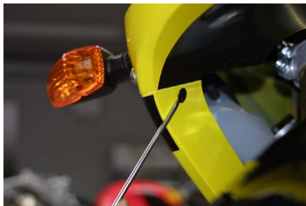
Figure 7: removal of the plastic pin
