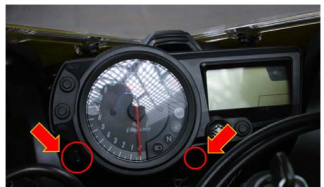
Figure 14: stock dash front screws position.
