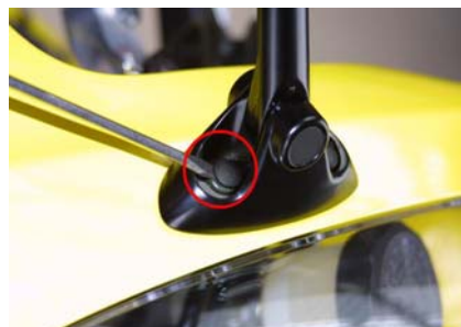
Figure 1: plastic covers removal.
