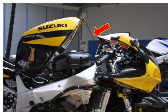
Figure 11: lifting the fuel tank
