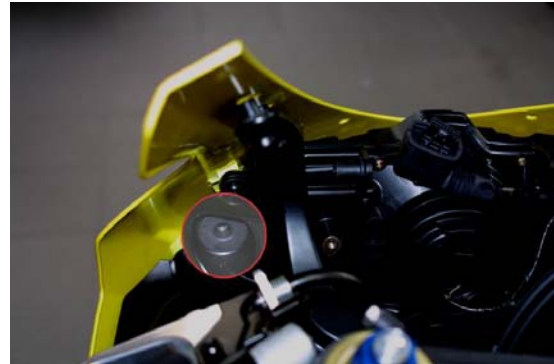
Figure 12: front fairing and high beam screws position
