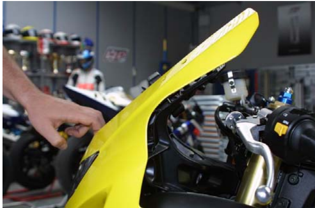
Figure 13: front fairing and high beam screws released.
