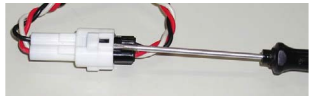
Figure 20: how to unplug a connector.
