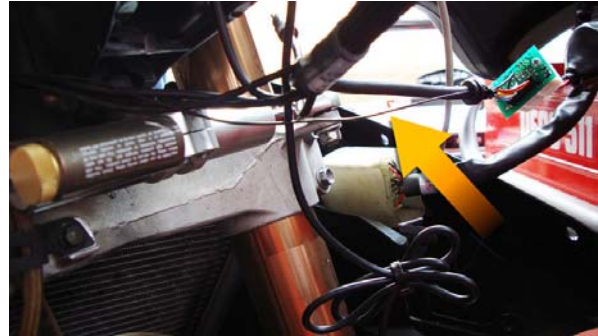
Figure 9: the ground black cable.
