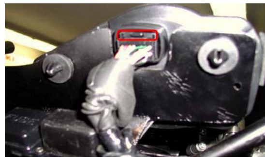
Figure 2: unplugging the 16 pins AMP connector from the stock dash.
