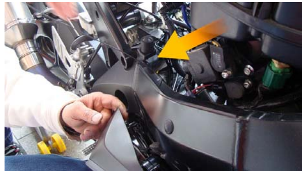
Figure 10: the ground cable runs along the chassis.
