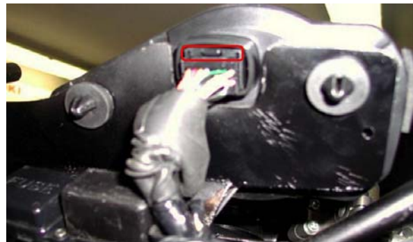
Figure 15: unplug the stock dash.
