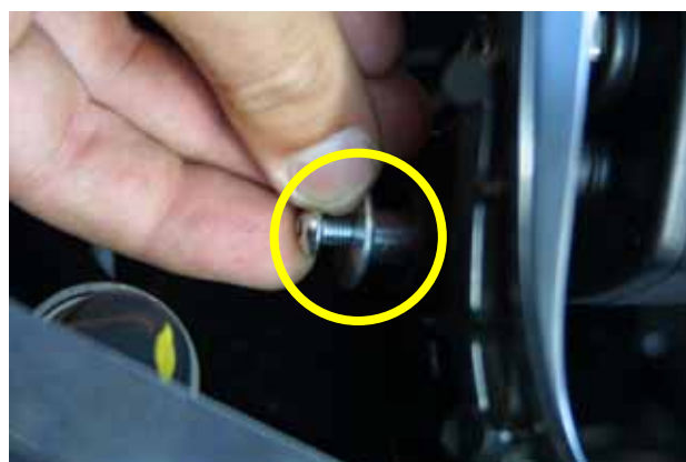
Figure 27: fixing MyChron 3 Plus / Gold to the bike.
