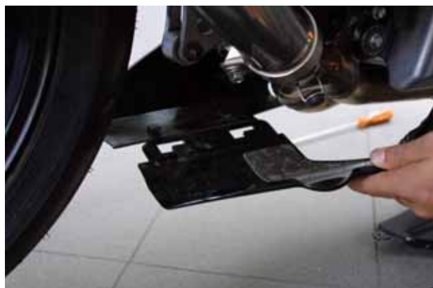
Figure 12: Slackening the groove of the lateral fairings
