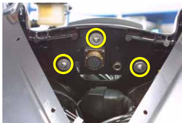
Figure 28: MyChron 3 correctly installed (rear view)
