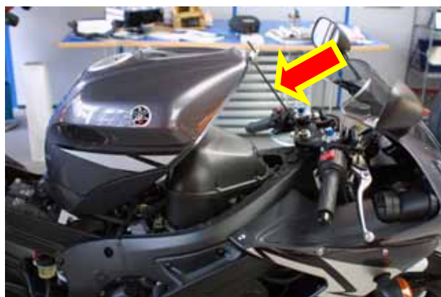
Figure 3:Uplifting the gas tank.
