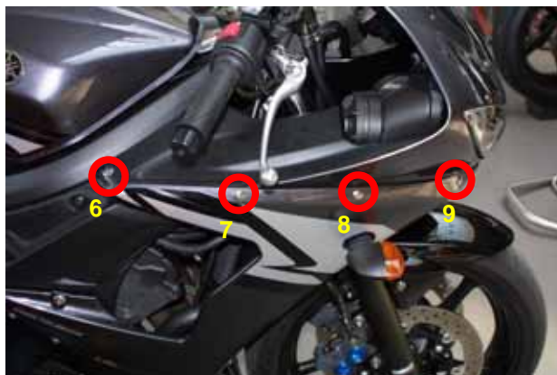
Figure 6: location of screws from 6 to 9
