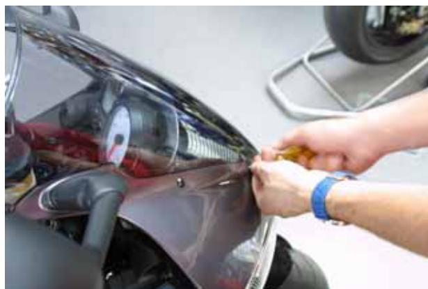
Figure 17: unscrewing the transparent fairing screws
