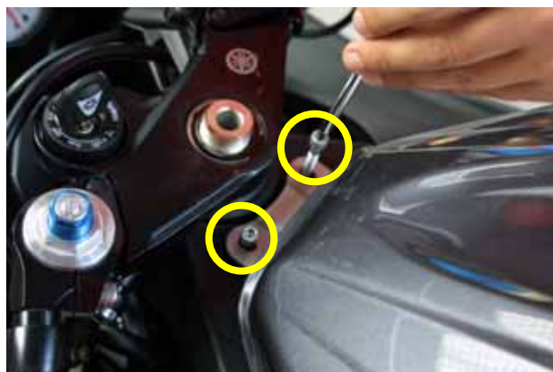
Figure 2: unscrewing the gas tank screws.
