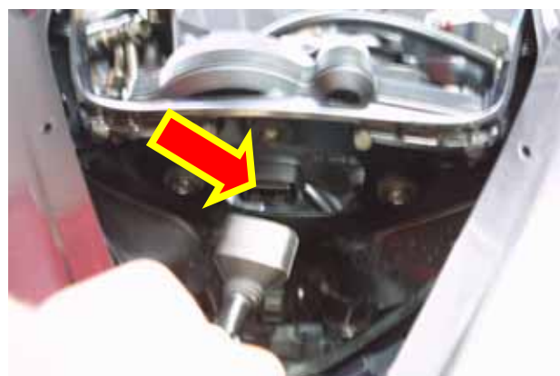
Figure 18: unplugging the on board dash connector
