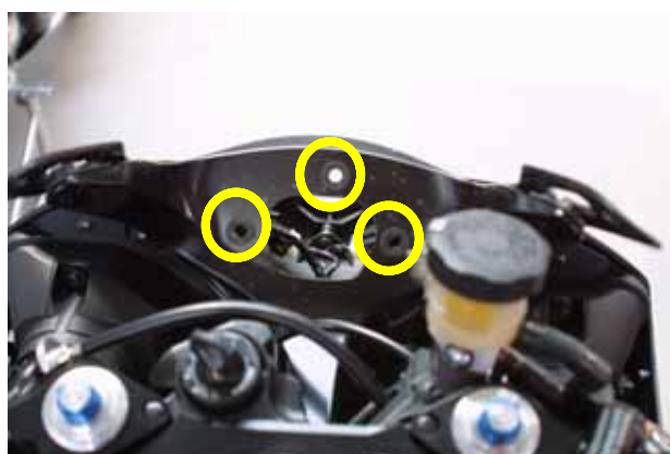
Figure 20: the stock dash has been removed
