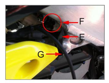
Make cable "G" of the image above on the right pass through the bike radiator, along the chassis as shown below on the left. Band it with the other cables highlighted below on the right.
