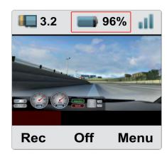
When battery level is too low a warning message appears for a few seconds on the display, the video itself closes and SmartyCam HD shuts down.
